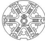
7-way trailer plug car end, rear view
